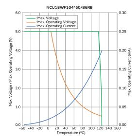
Max. Voltage, Max. Operating Voltage/Current Reduction Curve
