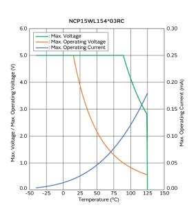
Max. Voltage, Max. Operating Voltage/Current Reduction Curve
