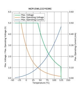
Max. Voltage, Max. Operating Voltage/Current Reduction Curve
