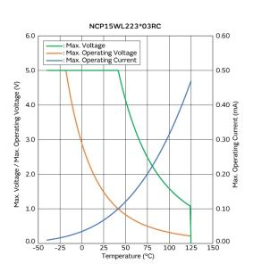
Max. Voltage, Max. Operating Voltage/Current Reduction Curve
