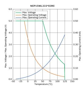
Max. Voltage, Max. Operating Voltage/Current **Reduction Curve**
