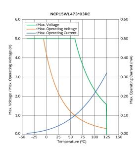
Max. Voltage, Max. Operating Voltage/Current Reduction Curve
