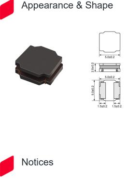
When rated current is applied to the products, inductance will be within ±30% of nominal inductance value. When rated current is applied to the products, the temperature rise caused by selfgenerated heat shall be limited to 40°C max. Keep the temperature (ambient temperature plus selfgeneration of heat) under 125°C.
