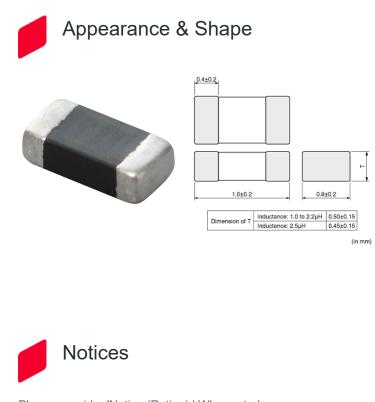
Please consider 'Notice (Rating).' When rated current is applied to the products, inductance will be within ±30% of initial inductance value range. When rated current is applied to the products, the temperature rise caused by self-generated heat shall be limited to 40°C max.
