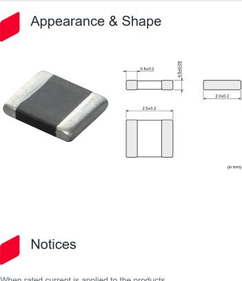
When rated current is applied to the products, inductance will be within  $\pm 30\%$  of initial inductance value range. When rated current is applied to the products, the temperature rise caused by selfgenerated heat shall be limited to 40°C max. Keep the temperature (ambient temperature plus selfgeneration of heat) under 125°C.
