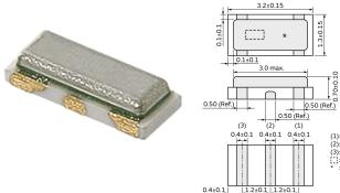
0.4±0.1 (1): Input (2): GND (3): Output Frequency Marking EIAJ Monthly Code (in mm) 1.2±0.1 1.2±0.1
