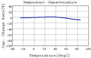
DE1B3RA221KN4APO1F C-Temp. capchange, DCOV,
