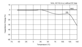
Capacitance - temperature characteristics
