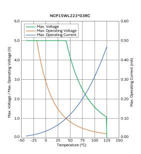
Max. Voltage, Max. Operating Voltage/Current Reduction Curve
