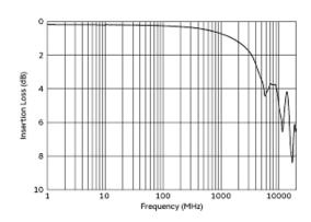
Common Mode Insertion Loss Characteristic (Typical Value)
