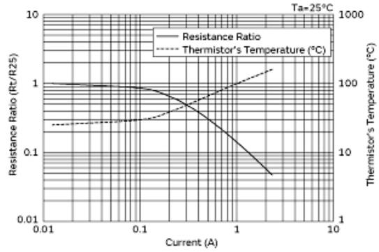
Current-R ratio (Rt/R25), Current-Temperature Characteristics
