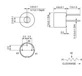
unit : mm Tolerance : ±0.3 Note: This datasheet may be out of date. Please download the latest datasheet of PV12P205A01B00 from the official website of Murata Manufacturing Co., Ltd.
