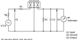
R1+Rg=R2=600 $\Omega$  ±5%, Rg=50 $\Omega$ C2=10pF (including stray capacitance and input capacitance of RF Voltmeter) E1: S.S.G. Output voltage
