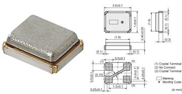
(1) Crystal Terminal (2) No Connect (3) Crystal Terminal Marking \* Monthly Code
