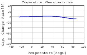
DE1B3RA681KN4APO1F C-Temp. capchange, DCOV,
