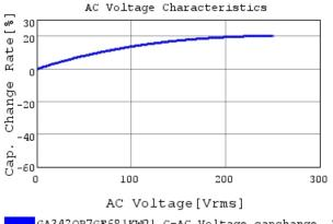
GA342QR7GF681KW01 C-AC Voltage capchange, D(
