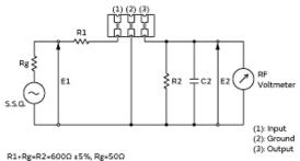
R1+R2+R2+B0001 25%, Rg=500 C2=10pF (including stray capacitance and input capacitance of RF Voltmeter) E1: S.S.G. Output voltage
