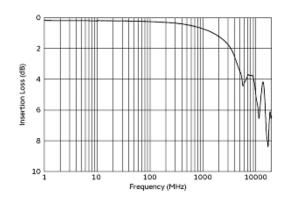
Common Mode Insertion Loss Characteristic (Typical Value)
