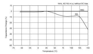
Capacitance - temperature characteristics
