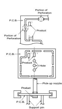
P.C.B. shall not be separated with hand. Suppor P.C.B. shall be separated with the fixture so as not to cause P.C.B. bending.
