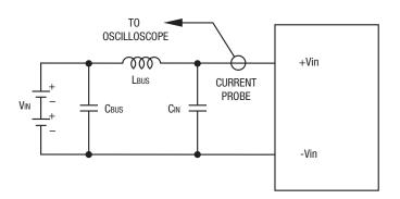
Figure 3. Measuring Input Ripple Current
