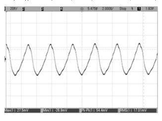
Output Ripple & Noise (Vin = 48V, lout = 35A, Cout = 1uF || 10uF, Ta = +25 $^{\circ}$ C)
