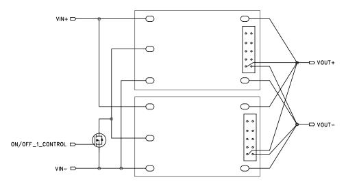
Figure 2. Load Sharing Block Diagram
