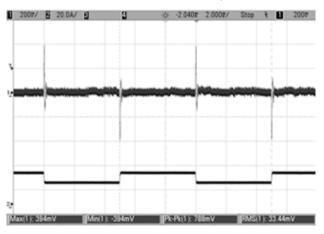
Output Ripple & Noise (Vin = 48V, lout = 0A, Cout =  $1 \text{uF} \parallel 10 \text{uF}$ , Ta = +25°C)
