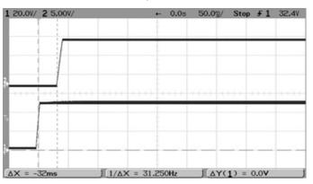
Stepload Transient Response (Vin = 48V, lout = 50-75-50% of lout, Cload = 1uF || 10uF, slew rate: 0.1A/us,  $Ta = +25^{\circ}C$ )
