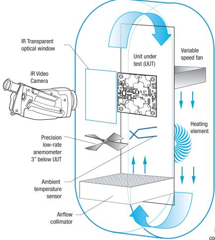
Figure 7. Vertical Wind Tunnel
