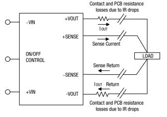
Figure 5. Remote Sense Circuit Configuration
