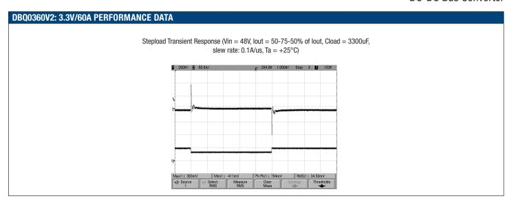
420W Digital Fully Regulated Intermediate DC-DC Bus Converter
