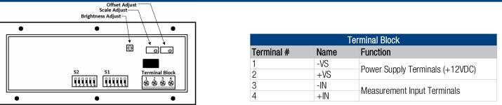
**Brightness Adjust** – This single-turn potentiometer supports adjustment of the meter's LED display brightness for maximum readability. Turning the pot clockwise increases brightness, while turning it counterclockwise decreases brightness.
