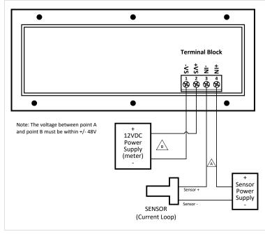
This example illustrates an application where the Current sensor is connected to terminals 3 and 4, where terminal 3 is the negative input terminal (-IN) and terminal 4 is the positive input terminal (+IN).
