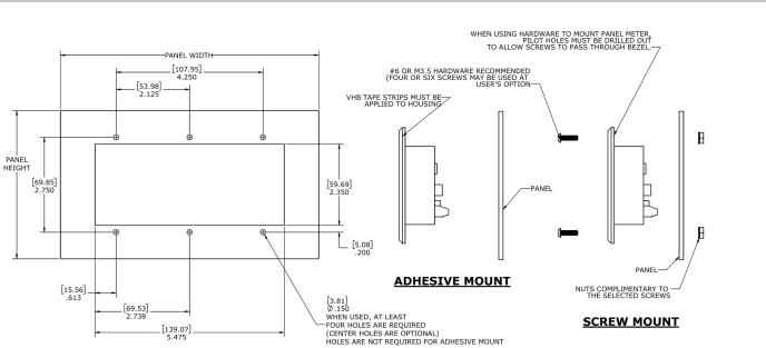
Note: When mounting panel meter with hardware, a four hole pattern (four outermost holes) or the six hole pattern may be used at the customer's option.
